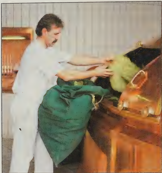
Hops being added to the brew in the kettle. The varieties are Brewers' Gold and Kent Goldings, but this is not intended to be a bitter beer.
